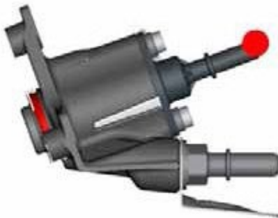
Figure 4-3 Measurement Location of DEF Dosing Module (Injector)
