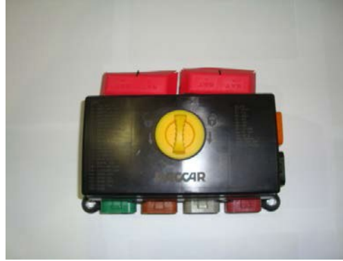
Figure 7.6.1 Pwer Distribution Center
