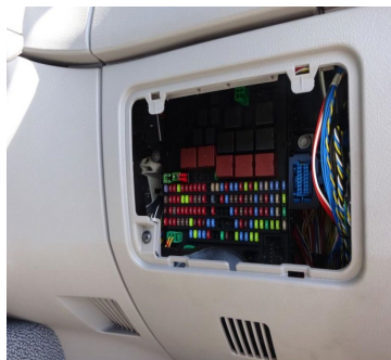
Figure 7-2.2 Inside View - Electrical Junction Box Location
