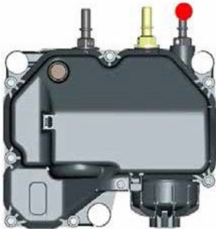
Figure 4-2 Measurement Location of DEF Supply Module (Pump)
